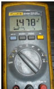
Utilizing my flex hands and arms, I reached the sensor on top of the fuel tank. By touching the connector, the voltage jumps from 4.3 to 1.4 volts. After replacing the FTPS and the pigtail, and by driving the car, all monitors set to ready with no problems.
