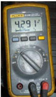
I decided to check the FTPS (Fuel Tank Pressure Sensor) signal at the PCM, and my voltmeter started to read 4.3 volts. According to FTPS testing procedure KOEO, the sensor should read around 1.5 volts.
