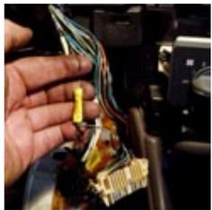
the IPC to the junction block as faulty. We removed the IPC. It looked OK but the wire was open so we started to unwrap the instrument cluster wiring harness. We found the MIL command wire had been cut inside the harness behind the IPC. The IPC side of the wire was spliced into an adjacent wire so the MIL appeared to work normally. The PCM control side of the wire was left open, and the harness was taped. That's why the PCM couldn't control the MIL.
