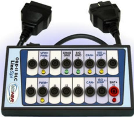
Attach one meter lead to Pin# 4 of the DLC and the other lead to battery negative with the engine cranking.
